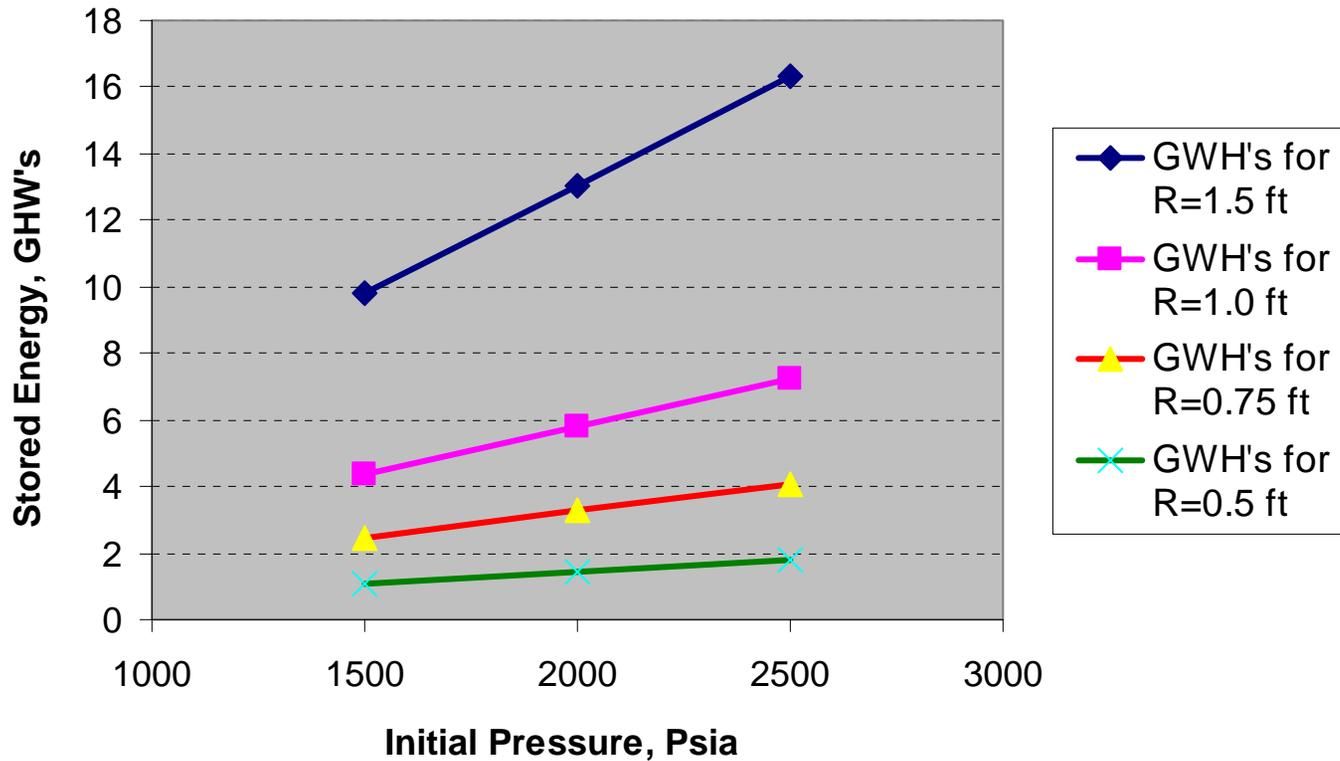
*The pipeline can store a tremendous amount of energy by operating between two different pressure levels.*
