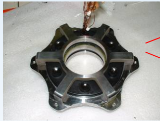
Magnetic Bearings – provide non-contact suspension of the rotor Texas A&M
