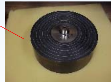
Composite Rotor – stores energy. Designed for long life, safety without containment, light-weight hubs, design and cert. standards
