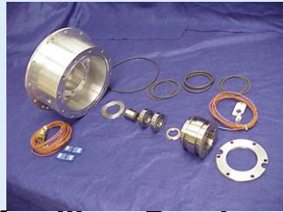
Auxiliary Bearings – carry launch and touchdown loads University of Toledo
