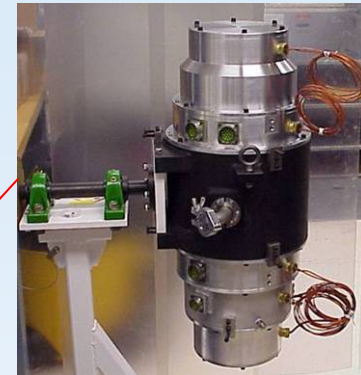
Housing – Lightweight aluminum housing provides spacecraft mechanical and thermal interface NASA Glenn/University of Toledo
